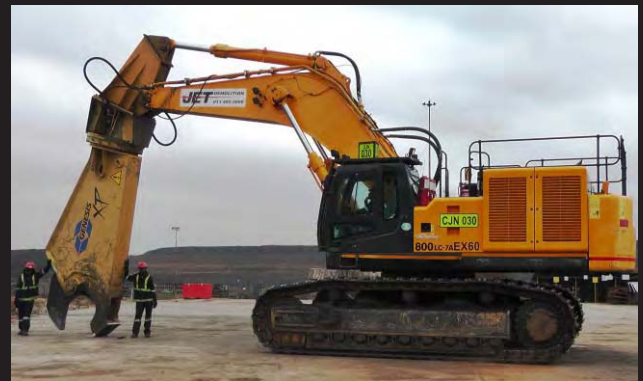
▲▲▲▲▲▲▲▲▲▲▲▲▲▲▲▲ 80 Tonne Demolition Excavator with a Large Specialised Demolition Shear
